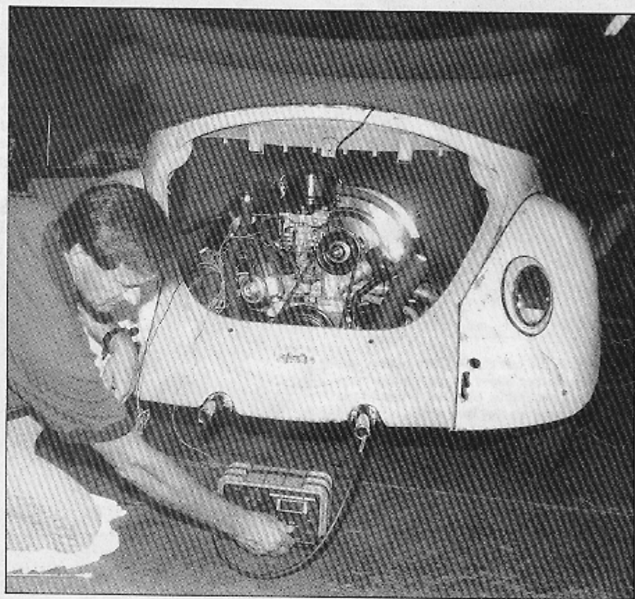
Tuning your engine to meet smog emission requirements has become increasingly important in nearly every state. We found the Gunson's Gastester Professional to be an accurate tool for determining the amount of Carbon Monoxide in the exhaust.
